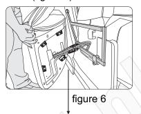
Note: the connect wire must be insert into the right place, avoid to get stuck.
