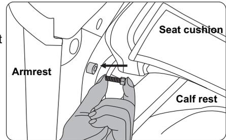
Figure: hex head screw fixed in behind part of armrest ( Figure 9)
