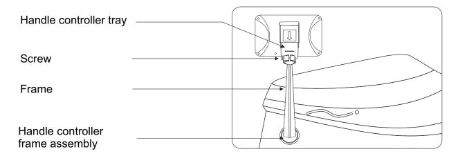
Ready for the handle controller tray, steel pole, take out the fixed screws on the handle controller tray. (Figure 1)
