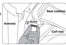
Figure: hex head screw fixed in behind part of armrest (Figure 9)
